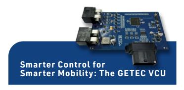
The Vehicle Control Unit (VCU) from GETEC is a powerful, flexible and scalable platform for the next generation of vehicles that adapts to various applications in electric, hybrid and intelligent vehicles.
